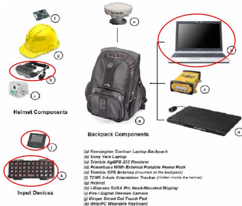
Figure 7.12 – Hardware Components of UM-AR-GPS-ROVER [Behzadan and Kamat, 2007]
