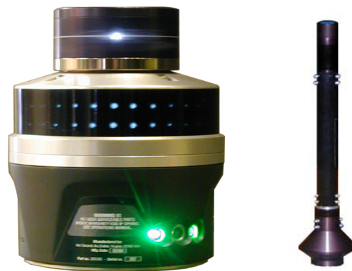
Figure 5.9 – Indoor GPS Transmitter (left) and Receiver (right) [Images courtesy of Dr. Kamel Saidi, NIST]
