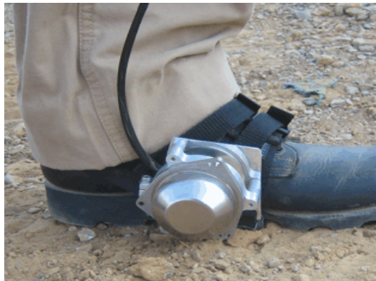
Figure 9.1 – Inertial Measuring Unit (IMU) mounted to the user's boot
