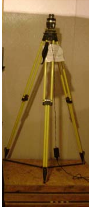
Figure A.13 – Transmitter Mounted on a Tripod
