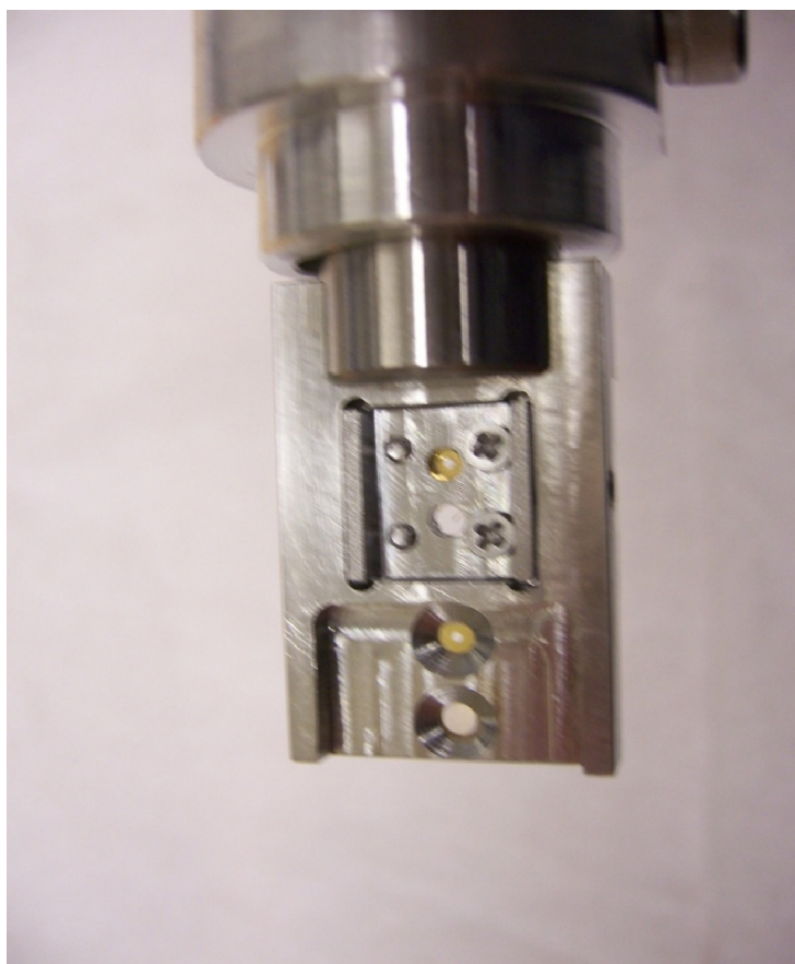
Figure 4-2 Rear view of sample holder with cartridge mounted. The bottom most aperture holds a gold 400M TEM grid; 5.0 mm above it is a gold 600 \mu\text{m} TEM aperture, and above that is the sample cartridge. Each of the TEM grid holder cells is centered on the same vertical line.
