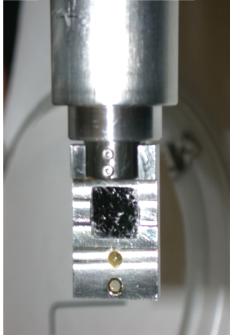
Figure 3-8 Sample holder with HOPG (highly ordered pyrolytic graphite) sample for reflection mode diffraction. Note the horizontal channel used for grazing incidence.
