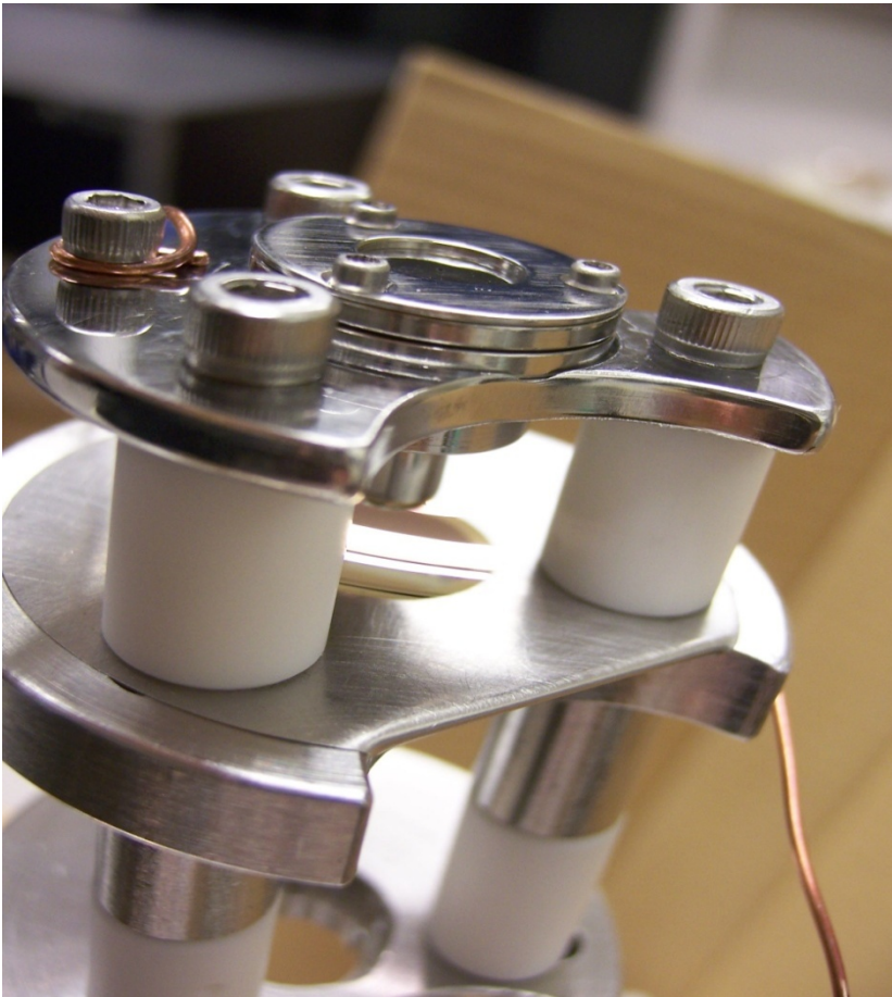
Figure 3-1 Photocathode and anode of the ultrafast electron gun, showing 30 kV electrical contact plate and 30 nm of gold sputtered onto a fused silica negative lens below; the grounded anode tube with 400M gold extraction grid leading up to a 200 um pinhole exit above. Operation requires an ultrahigh vacuum. The small bolts at the top are 0-80.
