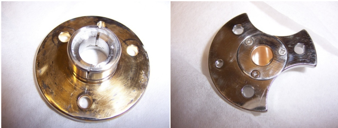
Figure 3-7 Left: Photocathode was held in a friction fitting. Right: Anode extraction grid was 500 LPI gold mesh.
