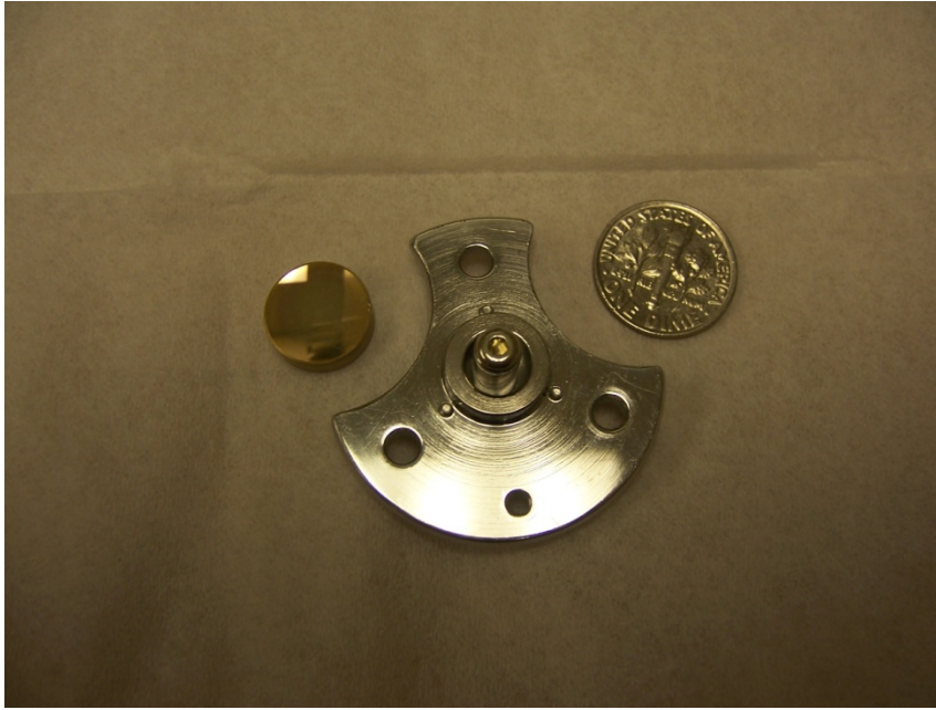
Figure 3-5 Anode structure, with photocathode at left. The cutaway sections allow for close passage of the pump laser beam and allow for a very close target sample.
