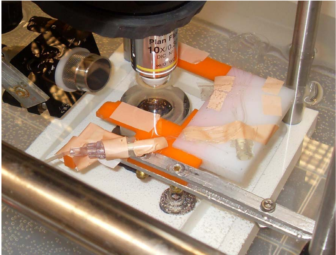
Figure 2.1a: Flow Tube Setup. (note: the hollow fiber of interest is barely discernible; the other 19 hollow fibers were taped onto the U-shape holder to prevent them from floating around in the tank)
