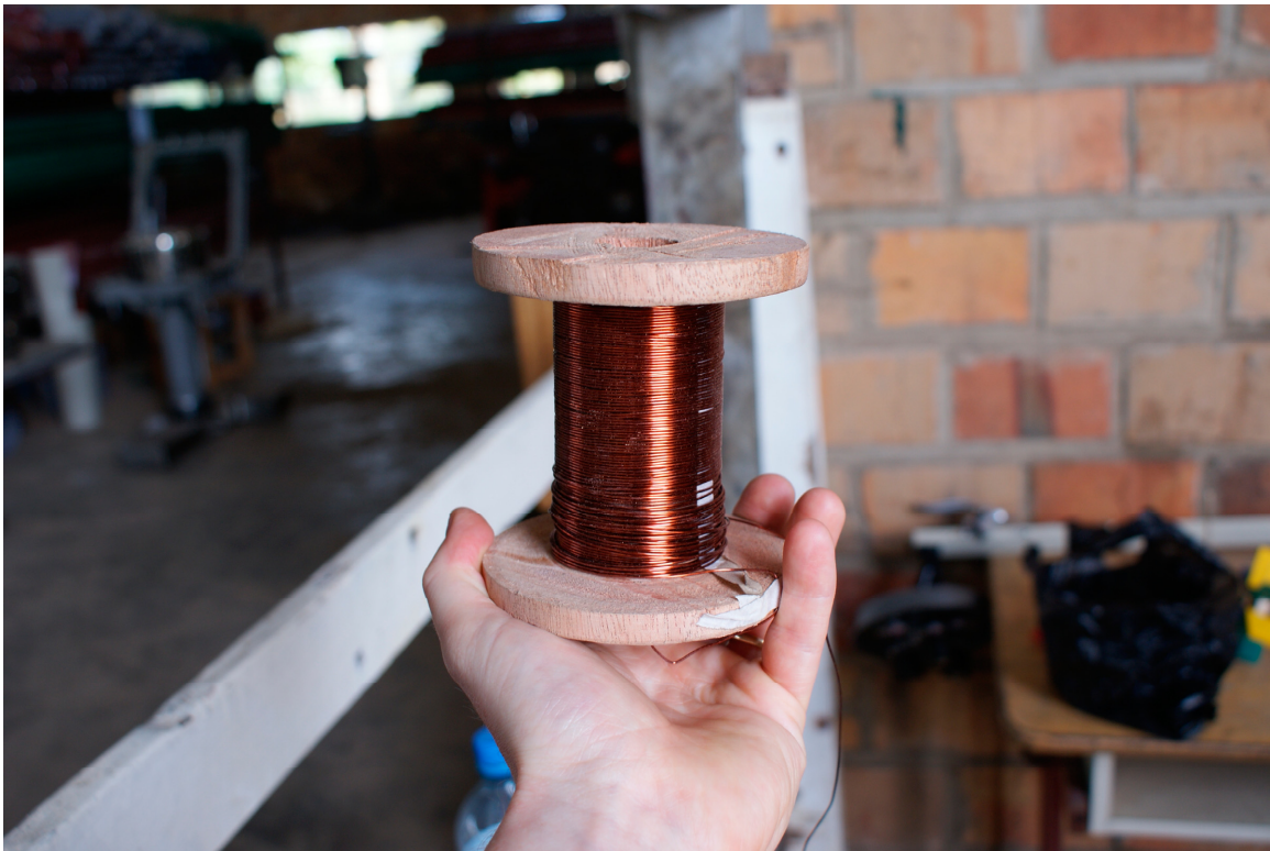
Figure 53: A handmade coil for one of the generators used on wind generator electrical device
