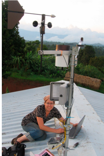
Figure 61: Hobo weather station being installed by me at Virika Hospital
