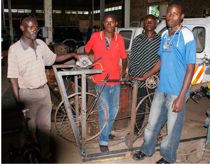
Figure 54: A triple geared hand-crank generator for surgical back-up lighting
