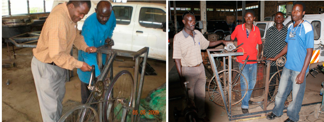
Figure 58: St. Joseph Technical Institute technicians' hand crank generator with bicycle DC permanent magnet motor used as generator (left) and with car alternator (right).
