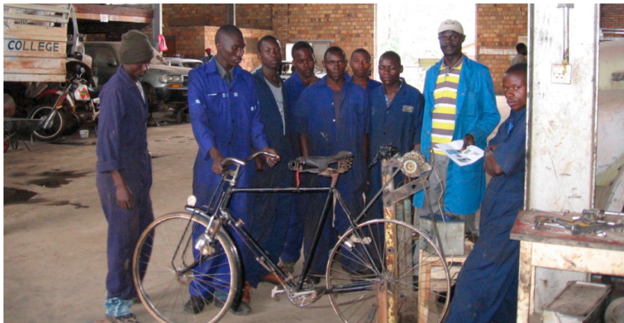
Figure 51: The final human bicycle generator produced at least 100 W. The multimeter wires began to melt and smell like burning rubber so we could not take an accurate measurement of the current.
