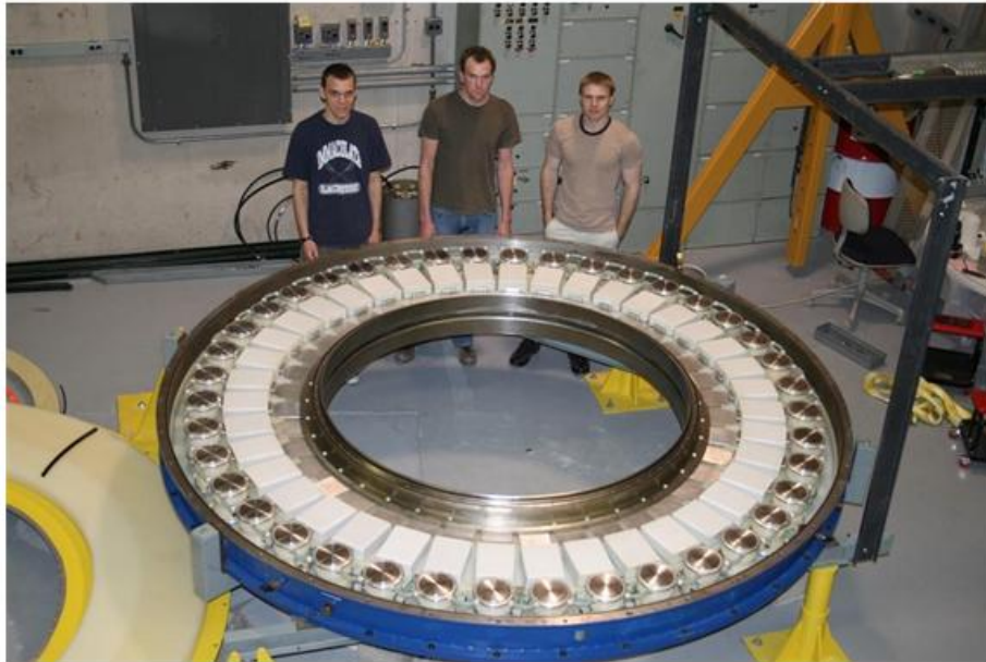
Fig. 1.5 A photograph of UM 1-MA LTD with connection of switches and capacitors shown [from Gil08].
