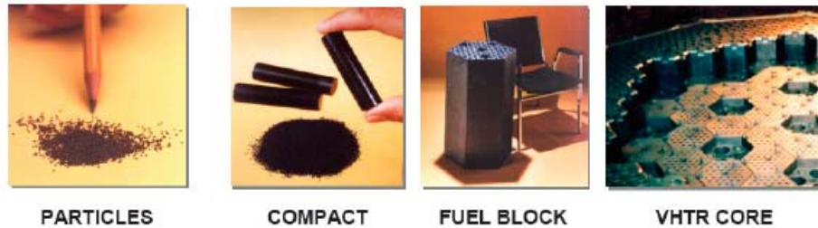
Figure 1.2. The construction stages of the prismatic VHTR core.
