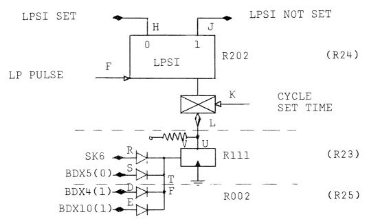
Notice that the LPSI is set by the LP PULSE and is cleared if bit 10 is set in control state instruction 62XX at CYCLE SET TIME. This allows the sense of the LPSI to be used to condition the skip logic in the same instruction that clears the LPSI.
