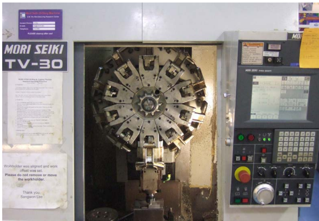
Figure 3-1 : FSW equipment by the use of Moriseiki CNC machining center
