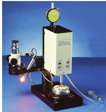
Figure 2.3: Model 170 Ultrasonic Disk Cutter from Fischione Instruments, Inc [Fis09].
