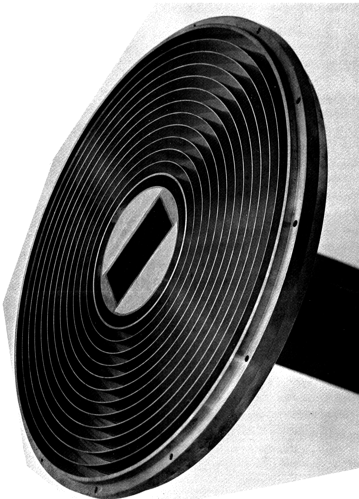
FIG. 2-1: SLOT ANTENNA AND CORRUGATIONS.
