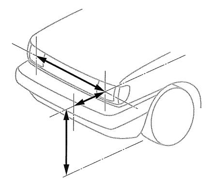
Figure 1. Schematic diagram of the three headlamp measurements taken for each vehicle.
