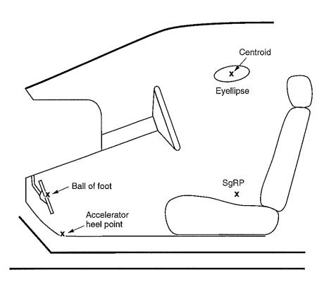
Figure 2. Schematic diagram of the relationship between the driver seating reference point (SgRP) and the mean driver eye position (the centroid of the eyellipse).
