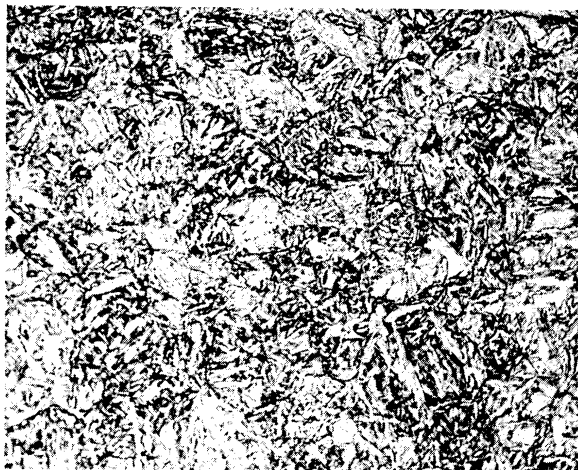
(c) Normalized at 2100°F + tempered 6 hrs at 1250°F + creep tested 1922 hrs at 1100°F and 30,000 psi - 240 BHN
