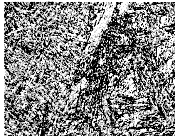
(b) Oil quenched from 1950°F + tempered 1 hr at 1300°F - 300 BHN
