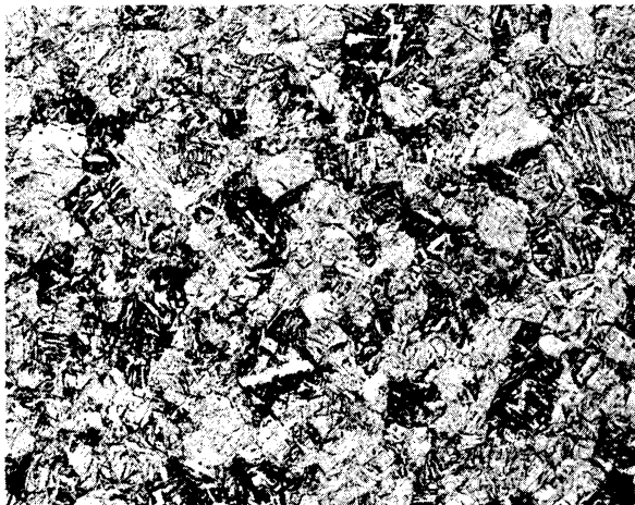
(b) Oil quenched from 1950°F + tempered 1 hr at 1300°F - 300 BHN
