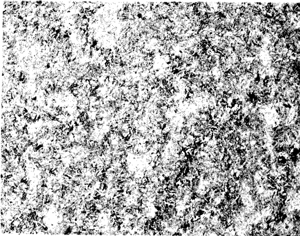
(a) Normalized from 1950°F as 3/4-inch Diameter Bar Stock - 435 BHN
