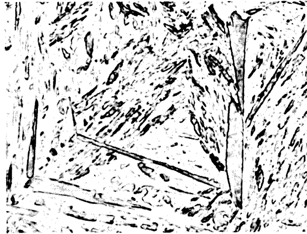
(a) Oil quenched from 2100°F As 1-inch Diameter Bar Stock - 534 BHN
