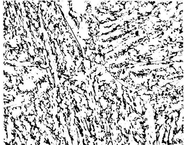
(a) Normalized at 2100°F as 1-inch Diameter Bar Stock - 312 BHN
