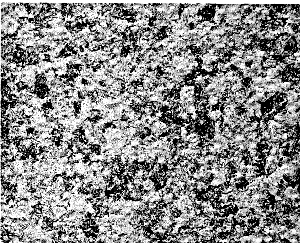
(c) Oil quenched from 1750°F + tempered 1 hr at 1300°F + creep rupture Tested 666 hrs at 1100°F and 20,000 psi - 265 BHN.
