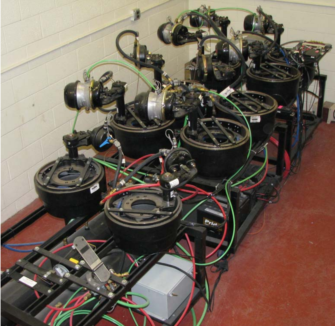
Figure 18. Physical Pneumatic Brake System With 10 Brake Actuation Chambers
