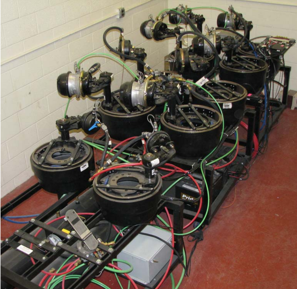
Figure 34. Physical Pneumatic Brake System With 10 Brake Actuation Chambers
