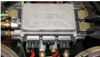
(c) trailer-axle package integrated with trailer ECU
