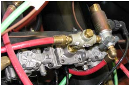
(a) front-axle package assembled with ESC solenoid valve
