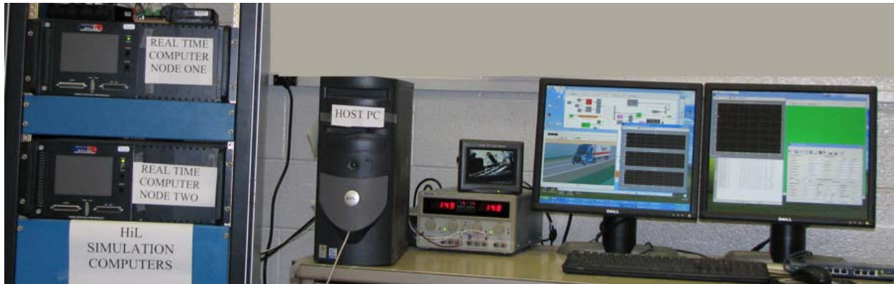
Figure 45. Physical Computer Setup for HiL Simulation
