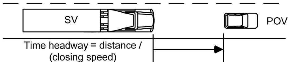
**Figure 11. QF1 Concept drawing: Time headway margin.**
