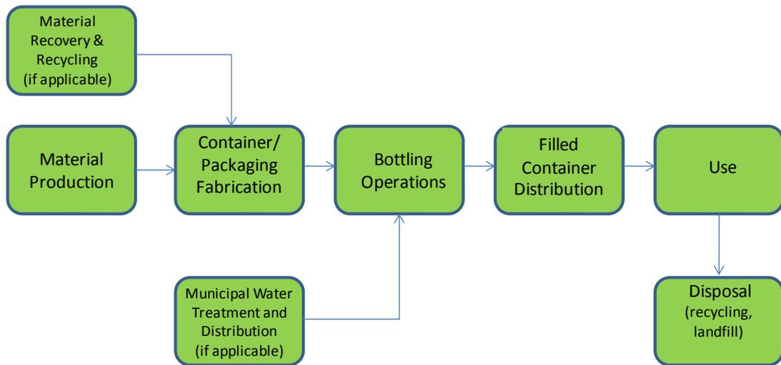
**Figure 2.1: Overview of Life-Cycle System Model**
