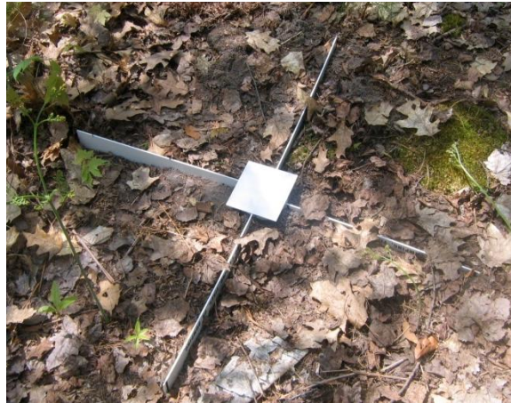
Figure 4. Pitfall trap made of plastic gates and buried container with glycerol.
