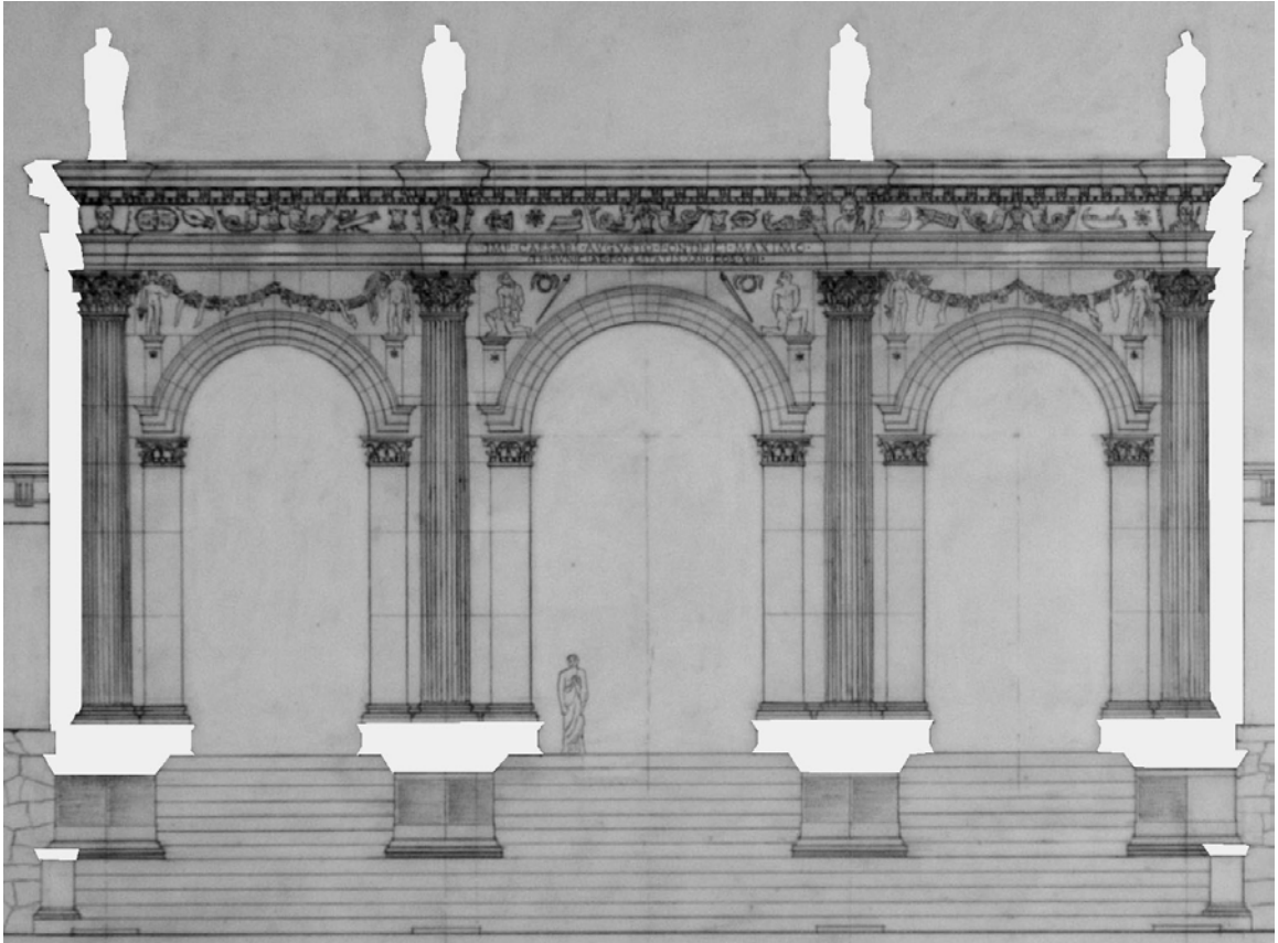
Figure 92. Diagram with the uncertain elements of Woodbridge's reconstructed elevation of the arch of Augustus blocked out. Illustration by the author.
