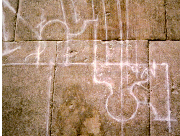
Figure 13: Detail of Molding Plans from Right Side of the South Tower Épure, Crypt of the cathedral, Bourges, France.
