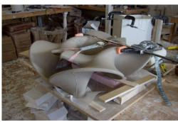
Figure 51: Evan Douglis, fLORA\_flex bricks being pieced together from slip-cast moulds.
