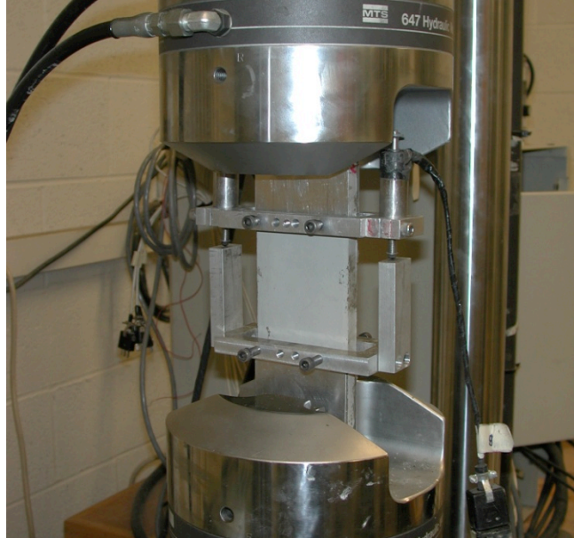
Figure 2.12 – Uniaxial tensile test setup.
