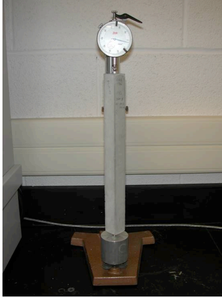
Figure 4.4 – Free drying shrinkage test.
