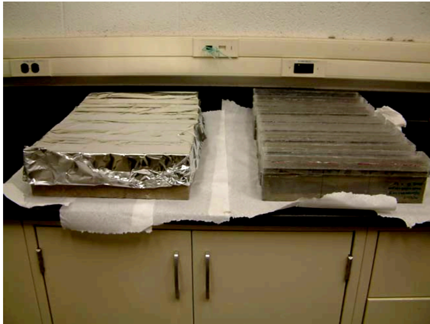
Figure 6.7 – Salt ponding test on uncracked and cracked beam specimens with dimensions of 355.6 mm x 50.8 mm x 76.2 mm (14 in. x 2 in. x 3 in.).
