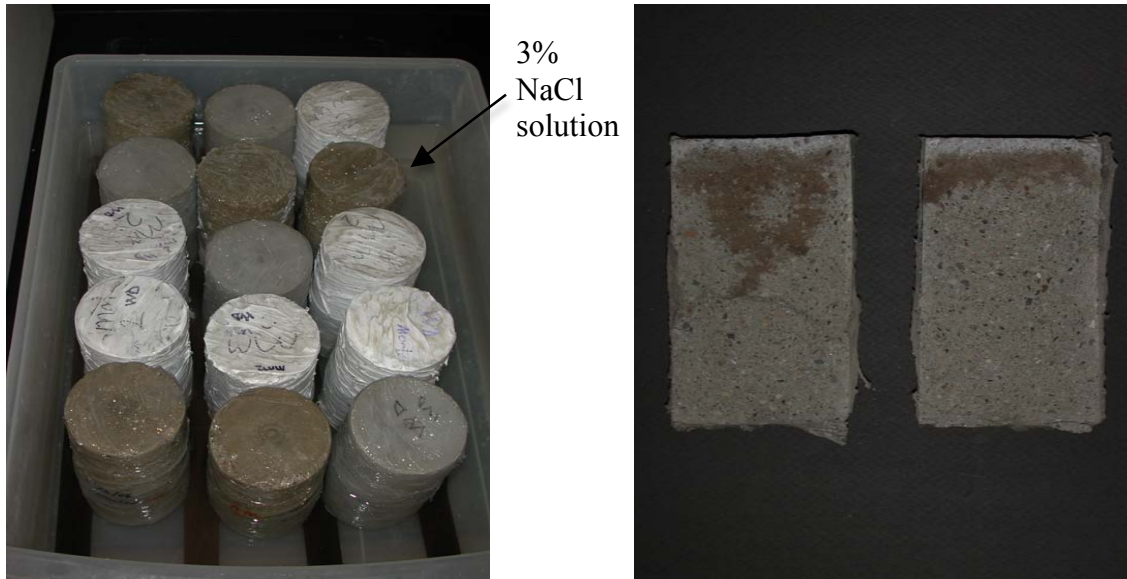
Figure 6.5 – Immersion test. (a) Cylinders were stored under continuous exposure to 3% NaCl solution. (b) One cylinder was taken out, split open, and sprayed with 0.1-N silver nitrate ( \text{AgNO}_3 ) solution, to measure the chloride penetration depth.
