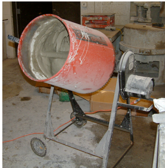
Figure 8.4 – Gravity mixer with capacity of two cubic feet (0.057 cubic meters).
