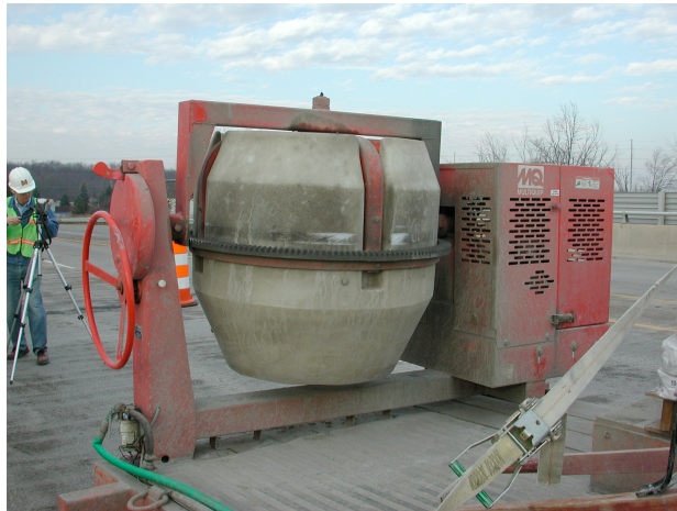
Figure 8.22 – 12 cubic foot (0.34 cubic meter) capacity gas mixer.
