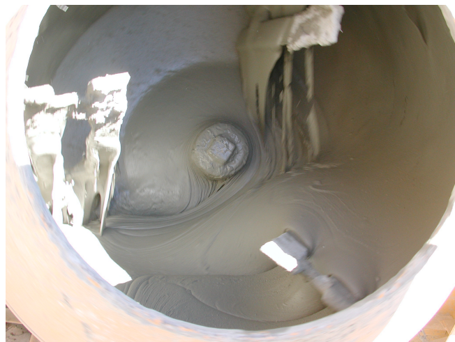
c) After adding cement (homogenous and creamy HES-ECC mortar matrix).
