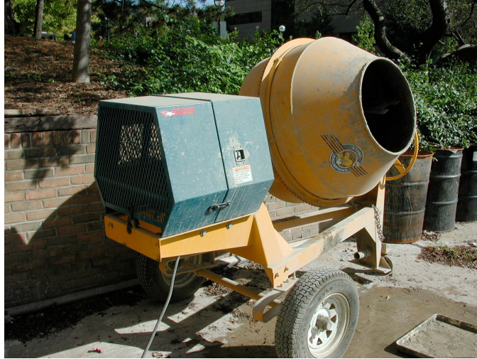
Figure 8.9 – Gravity mixer with capacity of 9 cubic feet (0.25 cubic meters).
