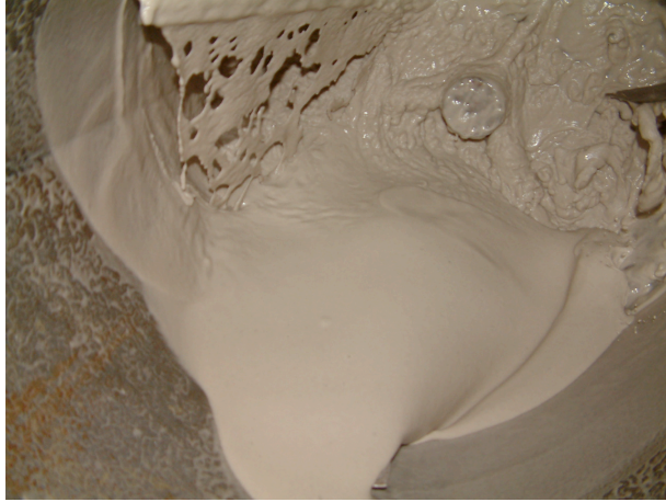
a) After adding sand, water, HRWR and hydration stabilizer.
