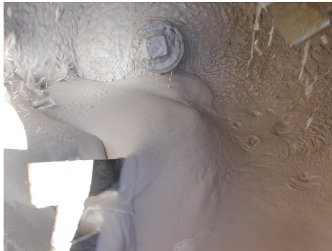
b) After adding sand, water, HRWR and hydration stabilizer.
