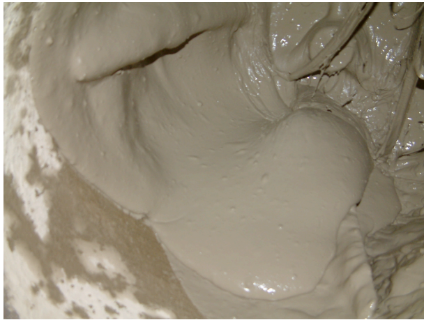
b) After adding cement (homogenous and creamy HES-ECC mortar matrix).
