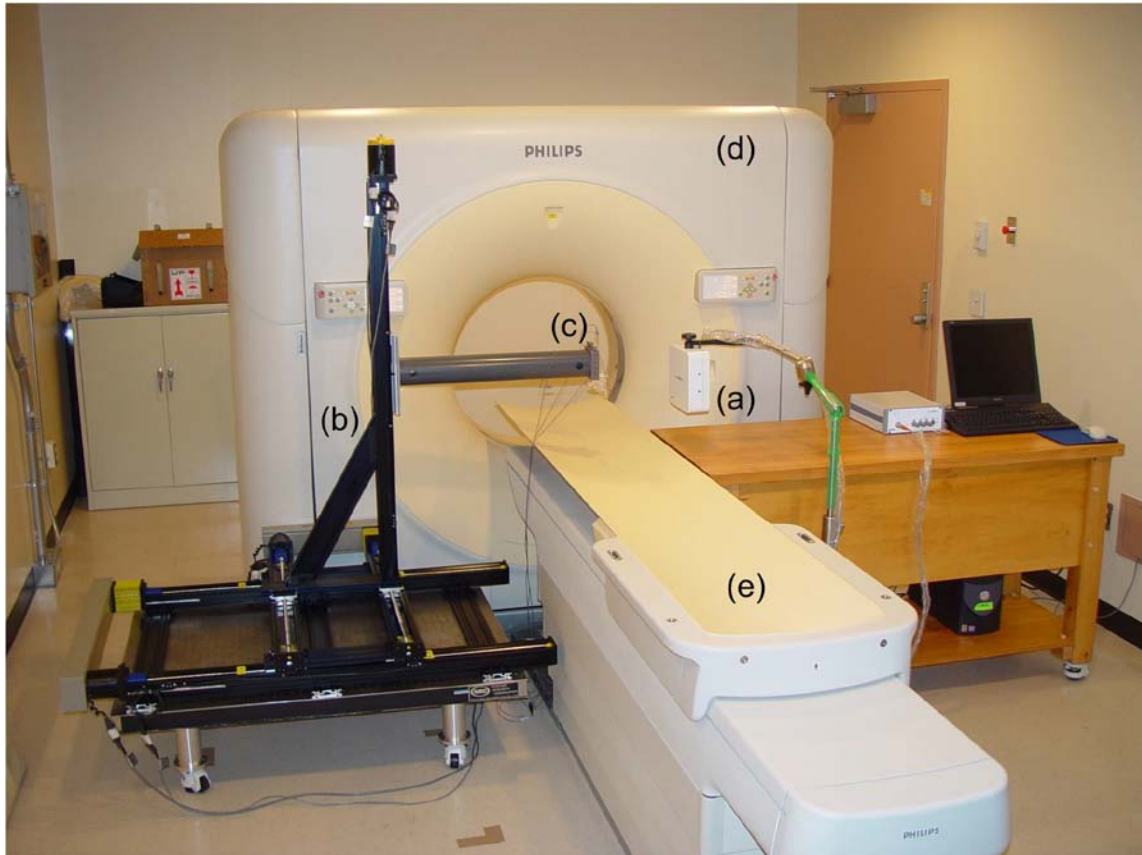
Figure 6.1: Setup of the CT scanner environment with a) NDI Aurora field generator besides the b) three-axis positioning system that raster scans the c) EM sensor holder. Also shown in the figure was the d) CT gantry and e) CT table.
