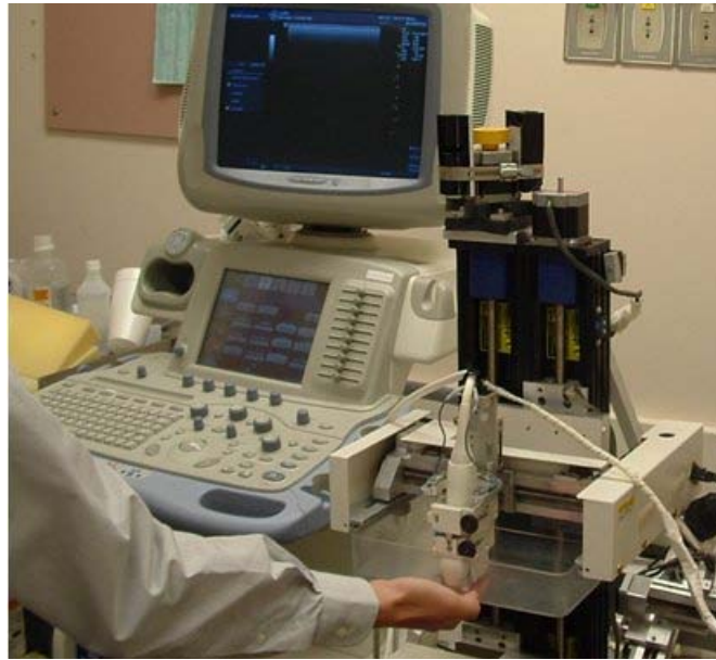
Figure 2.1: Experimental setup – apparatus to scan the finger and the TPX plate with the US scanner in the background. X and Y axes stepping motors for the transducer holders were on a frame attached to an upper compression paddle that helps stabilize the finger. Shown here, but not used in this study, are the vertical sliders and the bottom compression paddle.
