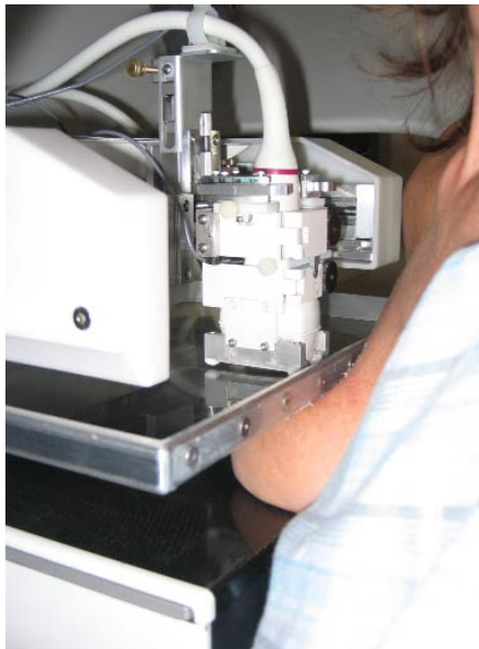
Figure 3.1: View of the breast under partial compression by mammography-style compression plates with the patient slightly rotated away in order to show the apparatus. Here, the transducer holder was spring-loaded in a frame attached to the paddle and moves above the compression plate with the transducer following the paddle surface. Notice that the transducer holder can be rotated about a vertical axis for scans at angles not parallel to the chest wall.
