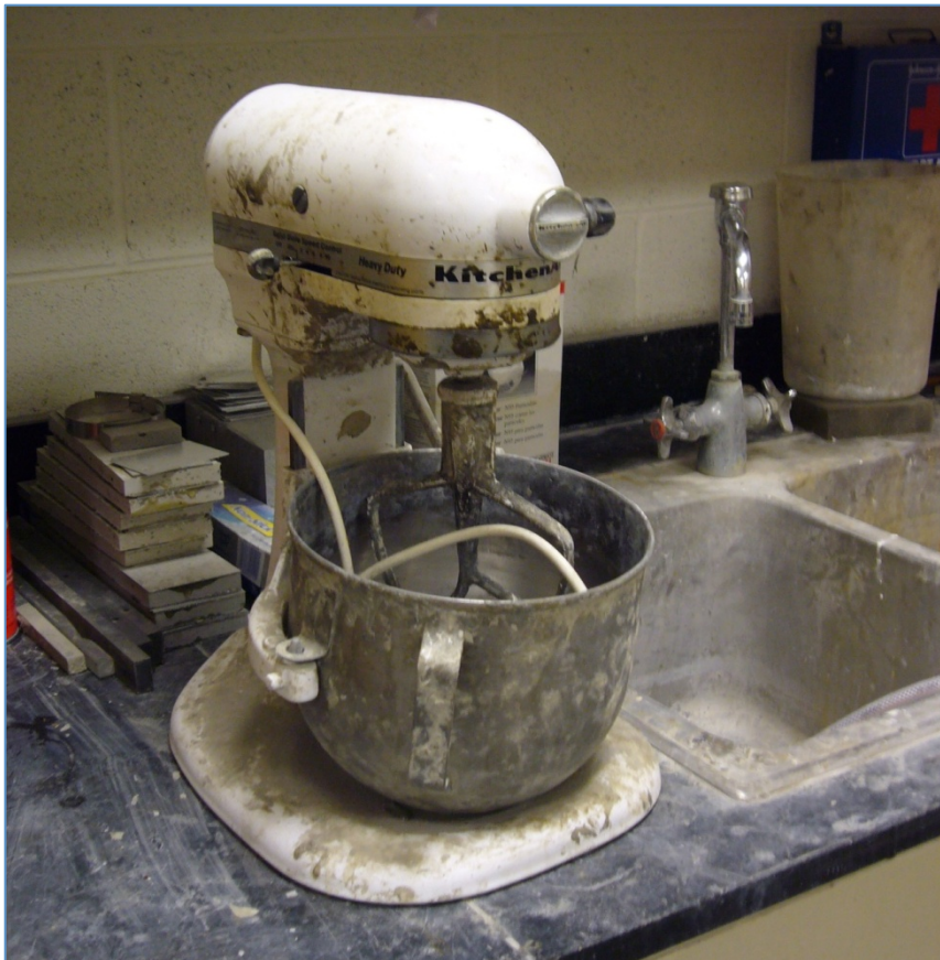
Figure 5-1. Blender used to mix most of MRL's ECC batches
