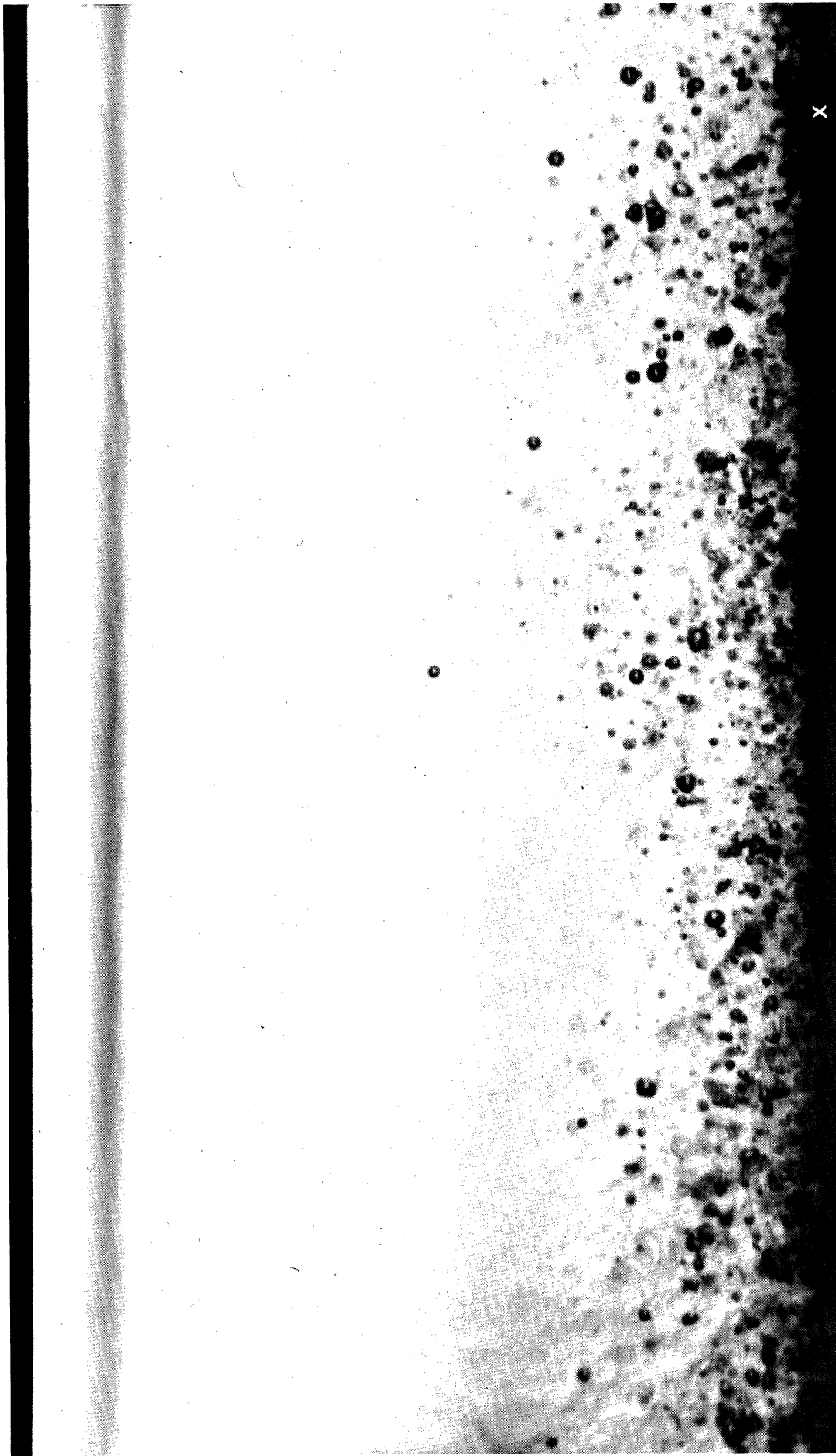
Figure 10. Still Photograph 19-9, before DNB, Scale = 16.8, P = 252 psia, \Delta T_{sc} = 106 \text{ }^\circ\text{F} , G = 3.01 \times 10^6 \text{ lb/hr-ft}^2 , q'' = 2.11 \times 10^5 \text{ Btu/hr-ft}^2 .
