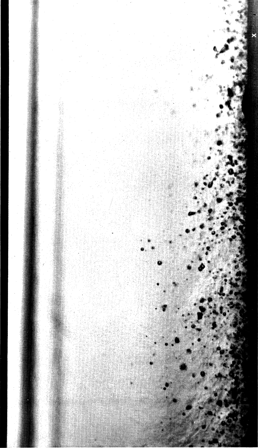
Figure 9. Still Photograph 19-8, before DNB, Scale = 16.8, P = 251 psia, \Delta T_{sc} = 106 \text{ }^\circ\text{F} , G = 3.01 \times 10^6 \text{ lb/hr-ft}^2 , q'' = 1.69 \times 10^5 \text{ Btu/hr-ft}^2 .
