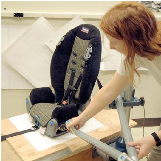
Figure 1. Digitizing child restraint geometry.
