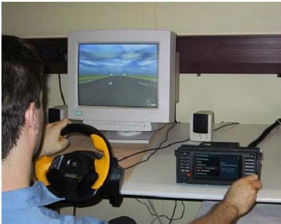
Figure 2. Setup of lane-change test using game controller
