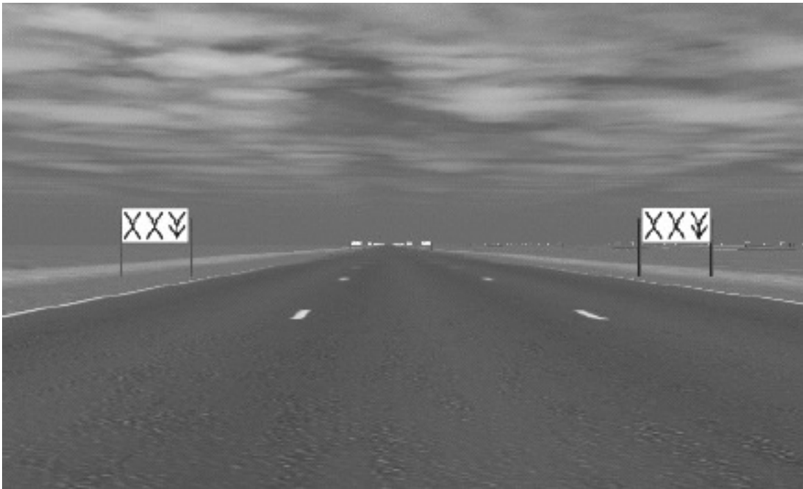
Figure 4. Lane change test road scene as per ISO indicating a change from the middle to right lane (Source: International Standards Organization, 2004)
