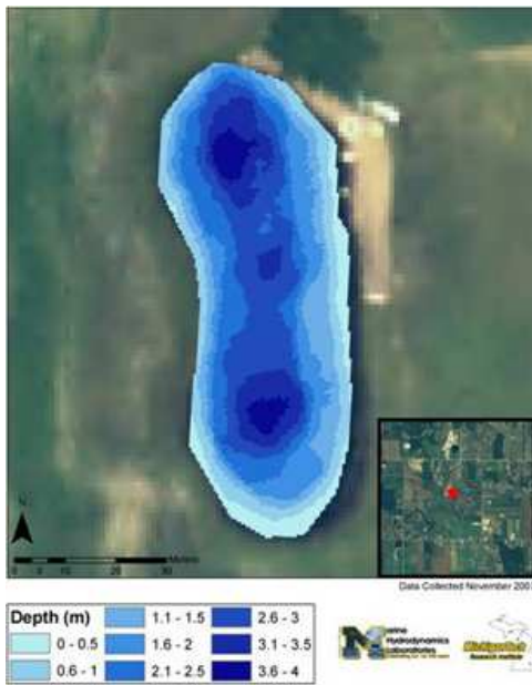
Fig. 8. Contour map of Wild Pond from bathymetry data.
