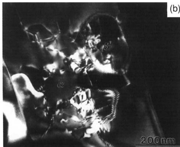
Fig. 6. (a) WB image of an elongated \beta' -SiAlON grain with twin boundaries and (b) complicated center region containing \alpha -Si 3 N 4 and a rounded supersaturated \beta' -SiAlON region.
