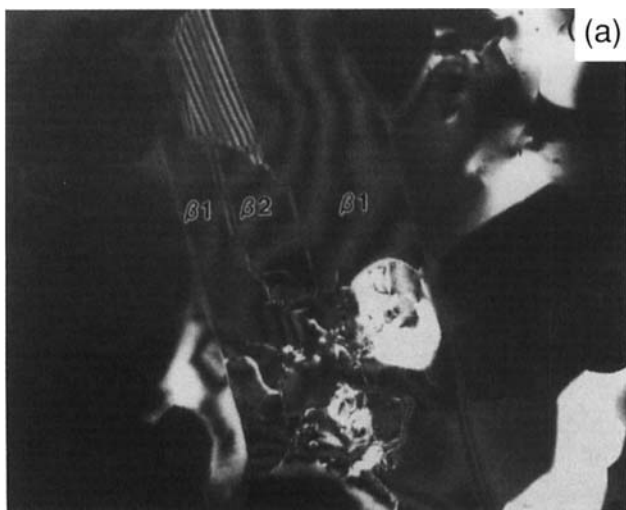
Fig. 6. (a) WB image of an elongated \beta' -SiAlON grain with twin boundaries and (b) complicated center region containing \alpha -Si 3 N 4 and a rounded supersaturated \beta' -SiAlON region.
