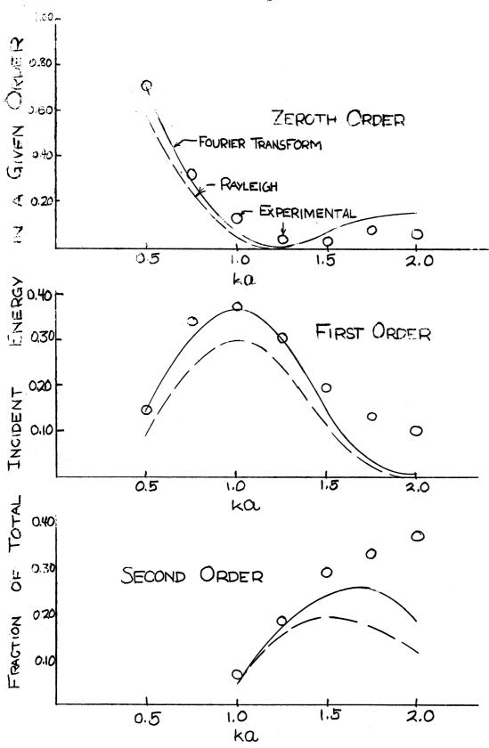
Figs. 3, 4, and 5. The figures show the energies calculated and observed in the zeroth, first and second diffracted orders reflected from a sinusoidal surface under the excitation of a normally incident plane wave; ax = 0.47.
