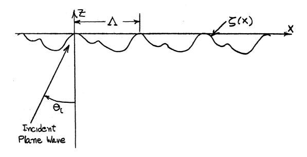
Fig. 2. The figure shows a plane wave incident upon a periodic surface.
