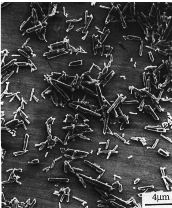
Fig. 1. Typical micrograph of the disintegrated grains of B10Y- \text{Si}_3\text{N}_4 ceramics. Sample was sintered at 1800^\circ\text{C} under 10-atm \text{N}_2 for 1 h.
