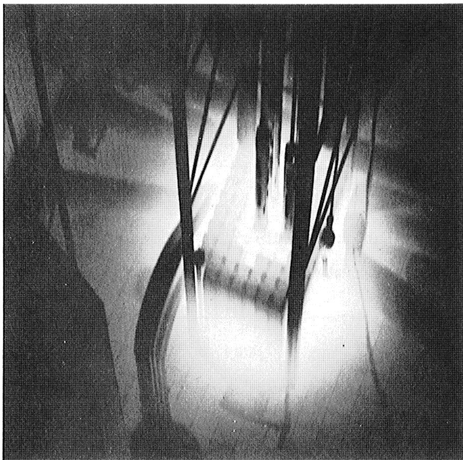
Figure 2. Reactor core at 100 kw; taken by its own light. Pneumatic tubes are at left of core.
