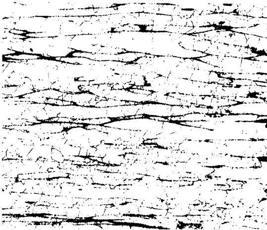
Figure 1 - Microstructure of Heat 201 Solution Treated 4 Hours at 1900°F Plus Aged 24 Hours at 1500°F, Aim Composition 0.01% B, 0% Ti.
