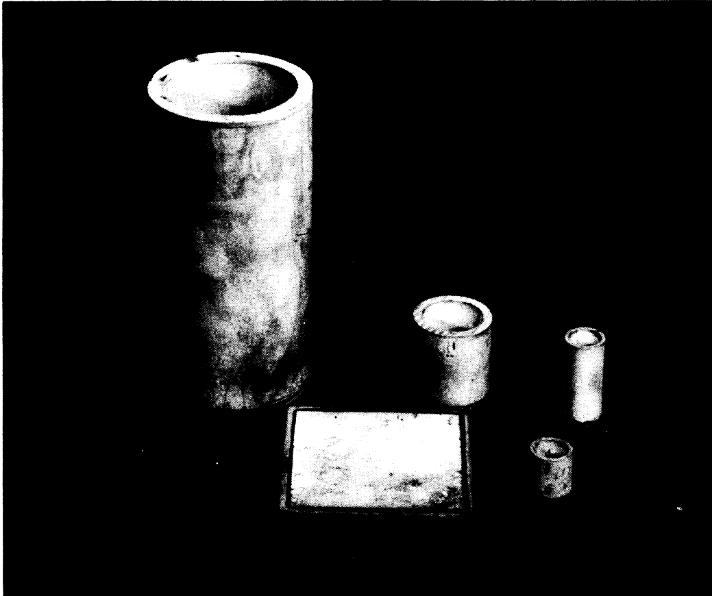
FIG.16 BASIC PIEZOELECTRIC CERAMIC ELEMENTS
