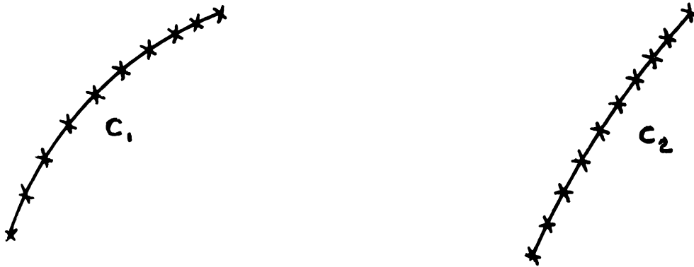
Figure 5. A given track as seen by the two cameras C_1 and C_2 . The cross marks represent measured points on the tracks.
