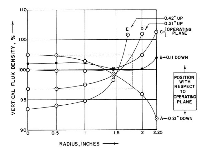
Figure 2. Test Results: Uniformity of Vertical Flux Density from Half-Helmholtz Coils, in the Operating Plane and at Other Levels.
