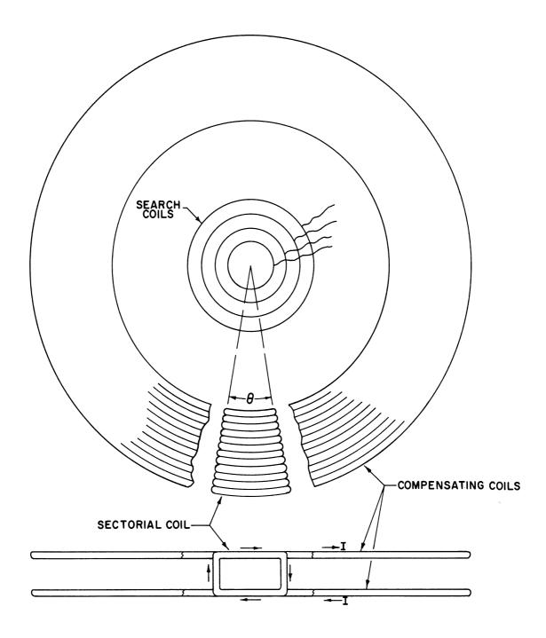
Figure 3. The Sectorial Coil, for Rapid Experimental Approach to Magnetic Lens Design. Experimentally, the Sectorial Coil Replaces the Complete Compensating Coils.
