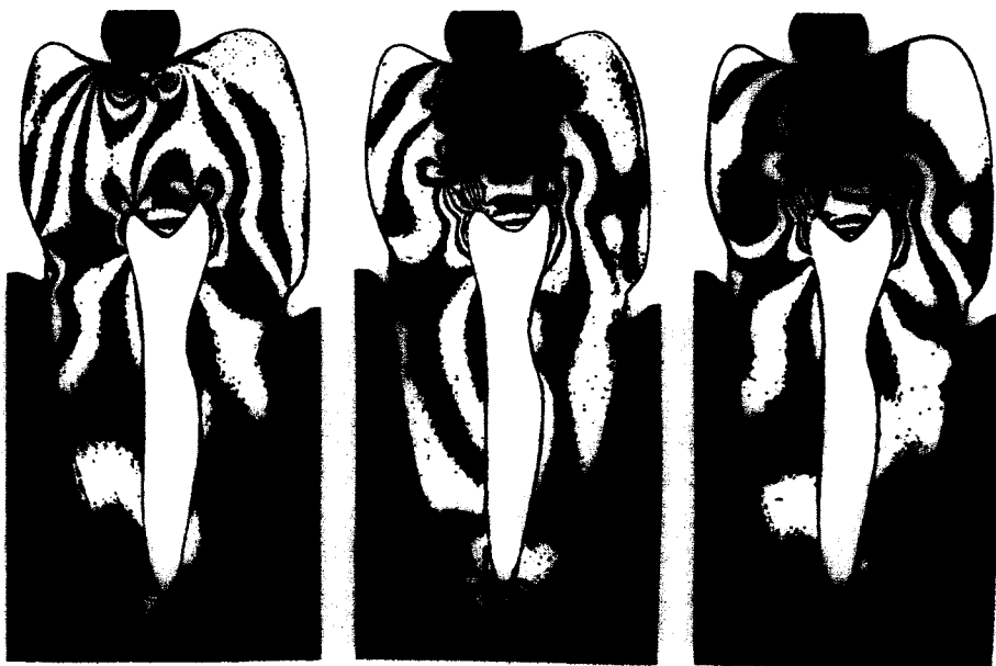
Fig. 3.—Stress distribution in a buccolingual section of a molar tooth subjected to an occlusal load for (A) a normal tooth, (B) one restored with an amalgam restoration, and (C) one restored with a gold inlay preparation.
