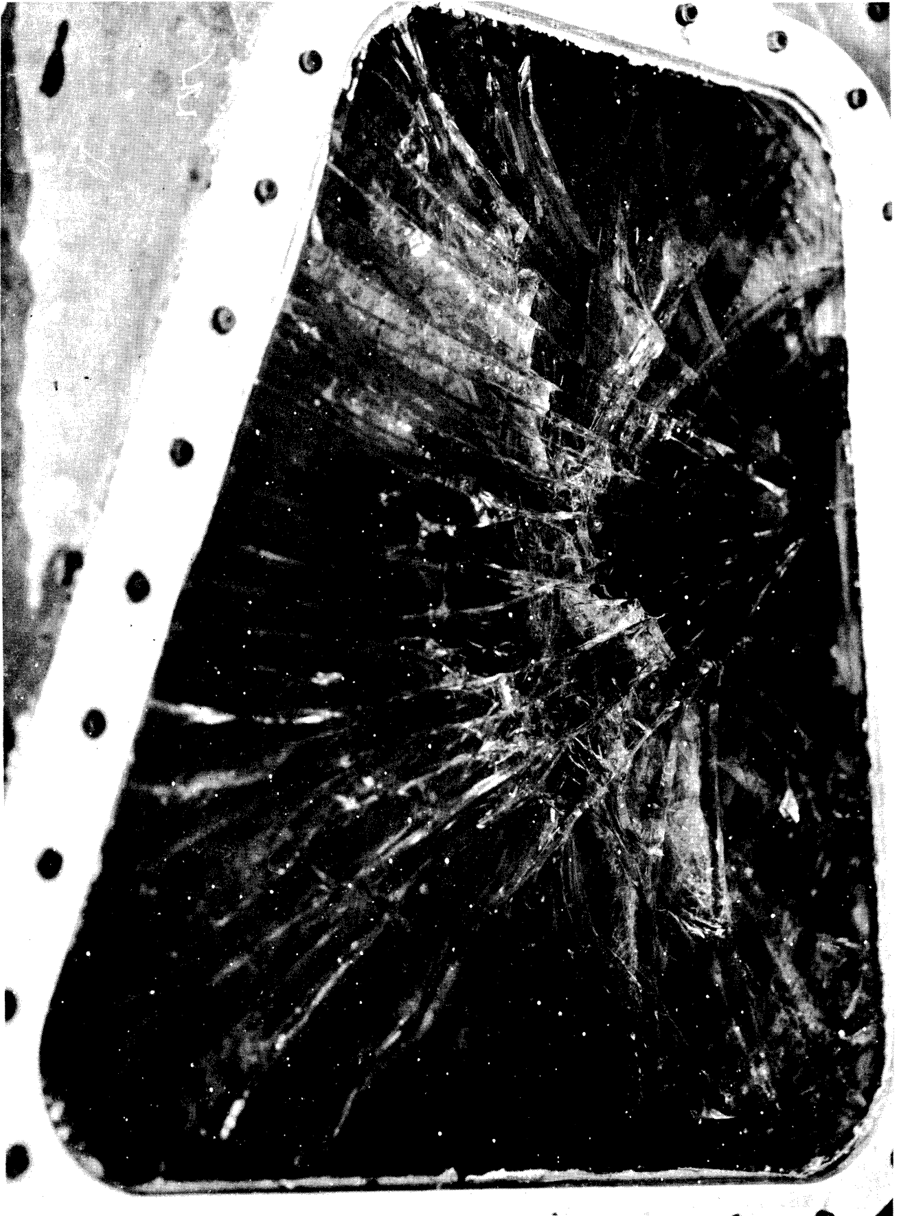
Figure 7. Uncoated commercial plate glass no. 2 after rupture.
