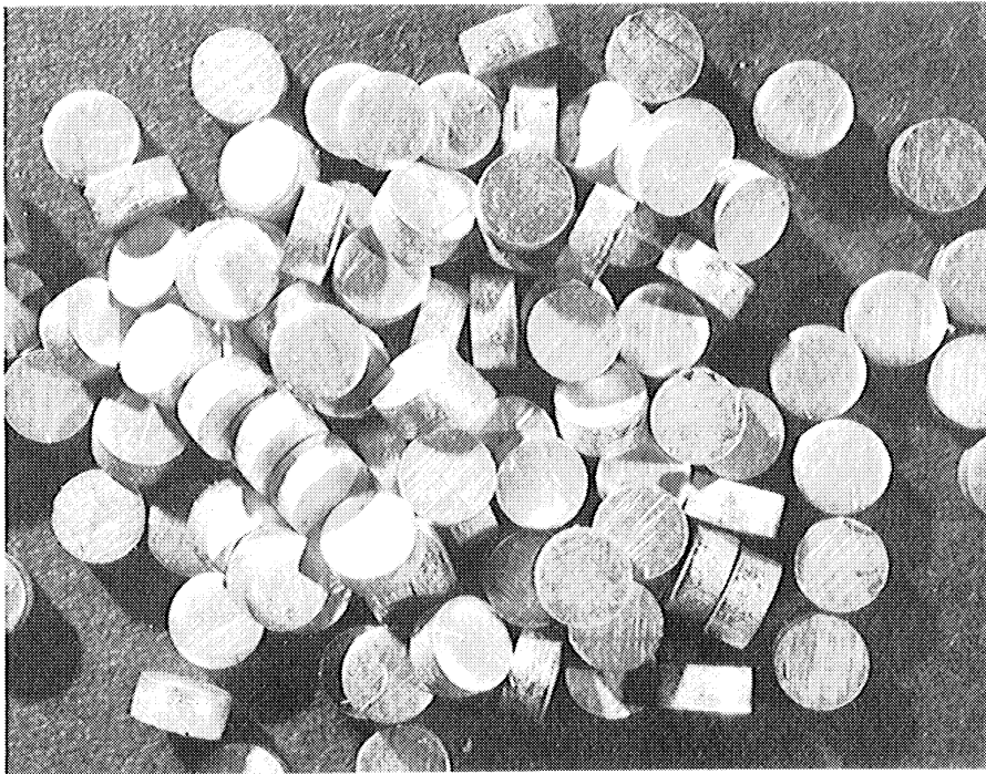
Figure 52. Flat Cylinders. (mag. approx. 4\times ) Laminated Aluminum.
