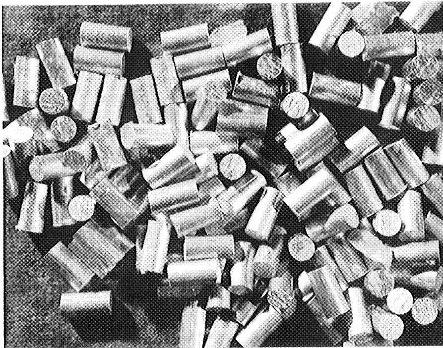
Figure 54. Long Cylinders. Aluminum Wire. (mag. approx. 4x)
