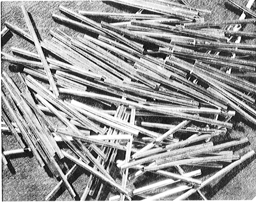
Figure 55. Needles. Copper Wire. (mag. approx. 4x)
