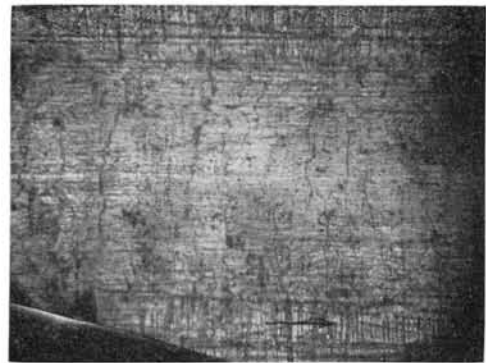
FIG 5.—Brittle behavior of amalgam at higher loads.
