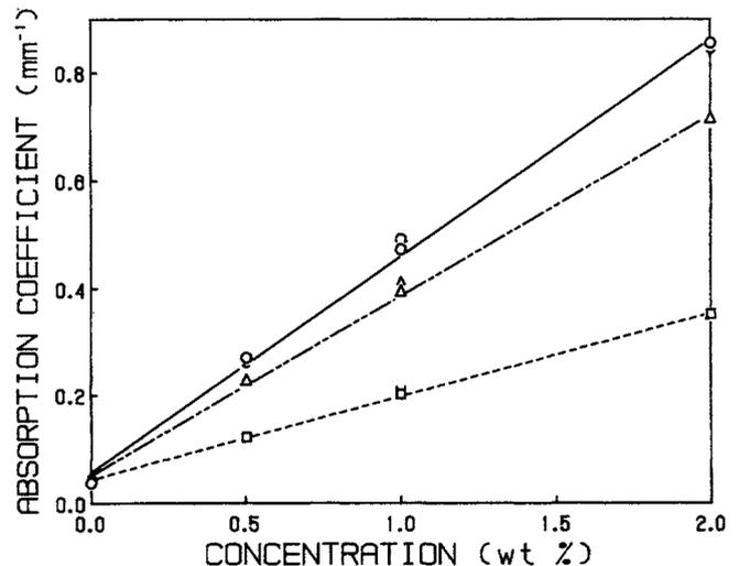
Fig. 6 — Scatter diagrams and regression lines for Kubelka-Munk absorption coefficients vs. concentration at 450 (open circles and solid line), 550 (open triangles and long-short-short dashed line), and 650 nm (open squares and dashed line) for red brown flockings.
