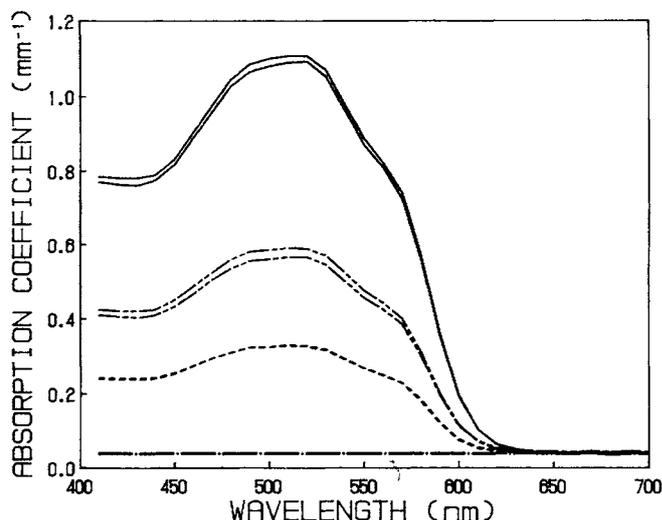
Fig. 1 — Spectra of optical absorption coefficients for maxillofacial elastomer with red flocking in concentrations of 2.0 wt% (solid line), 1.0 wt% (long-short-short dashed line), 0.5 wt% (dashed line), and 0.0 wt% (dash-dot line).
