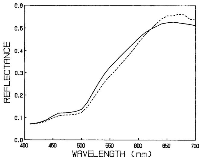
Fig. 7 — Spectra of calculated (dashed line) and observed (solid line) reflectivities for dark buff dry mineral earth pigment at 0.10 wt%.
