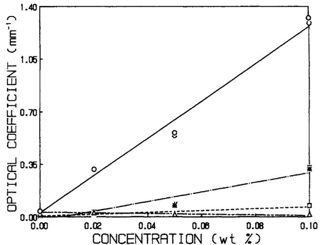
Fig. 5 — Scatter diagrams and regression lines for Kubelka-Munk absorption (K) and scattering (S) coefficients vs. concentration at 450 nm (K, open circles and solid line; S, open squares and dashed line) and 550 nm (K, open triangles and long-short-short dashed line; S, \* and dash-dot line) for yellow dry mineral earth pigment.
