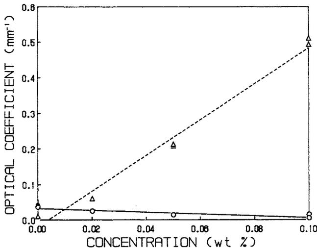
Fig. 3 — Scatter diagrams and regression lines for Kubelka-Munk absorption (open circles and solid line) and scattering (open triangles and dashed line) coefficients vs. concentration at 550 nm for titanium dioxide.
