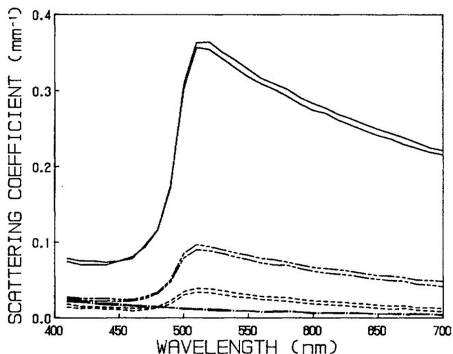
Fig. 2 — Spectra of optical scattering coefficients for maxillofacial elastomer with yellow dry mineral earth pigment in concentrations of 0.10 wt% (solid), 0.05 wt% (long-short-short dashed line), 0.02 wt% (dashed line), and 0.00 wt% (dash-dot line).
