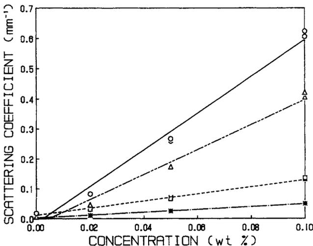
Fig. 4 — Scatter diagrams and regression lines for Kubelka-Munk scattering coefficients vs. concentration at 450 and 650 nm for titanium dioxide (450 nm: open circles and solid line; 650 nm: open triangles and long-short-short dashed line) and white dry mineral earth pigment (450 nm, open squares and dashed line; 650 nm, \* and dash-dot line).
