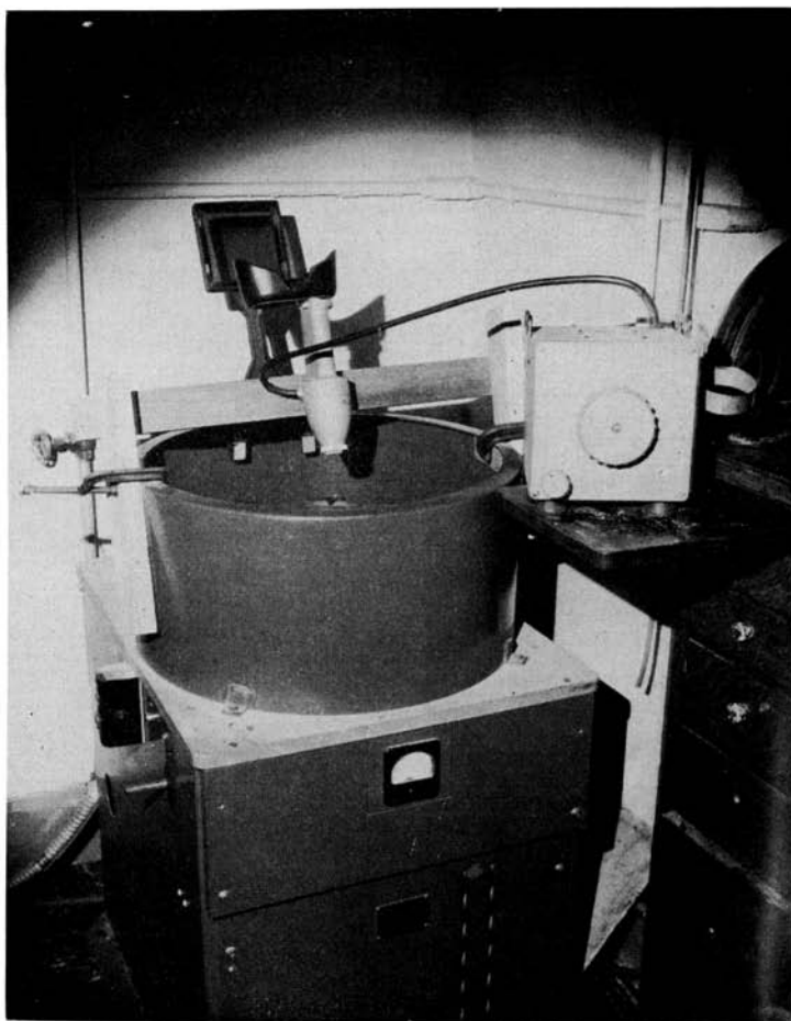
FIG. 3.—Williams casting machine and optical pyrometer
