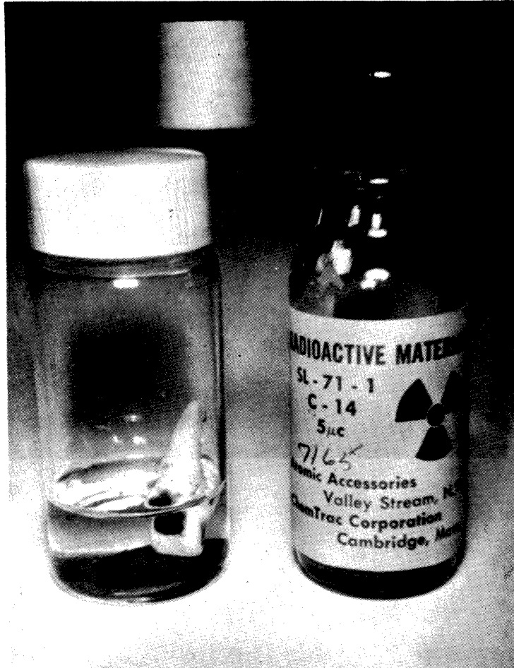
Figure 8. Tooth Immersed in Radioactive Solution for Penetration Tests.
