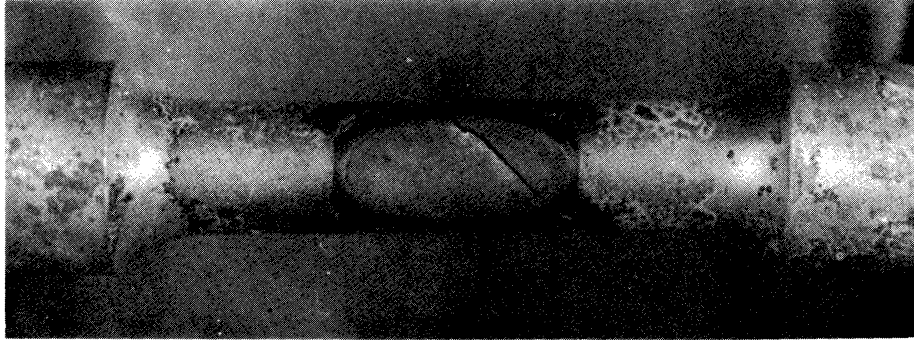
Zincified S35C test piece, \tau_a=15.0 \text{ Kg/mm}^2 , h=0.5 \text{ mm} , N=1.95 \times 10^6
