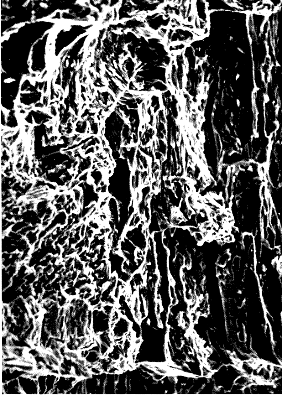
Figure 12. Scanning electron micrograph of a fracture from a 6" Y block which exhibited a gas test pressure of 61 mm Hg. The higher elongation of 11% provides a mixture of cleavage and shear failure. (Compare to Fig. 11). 500X.
