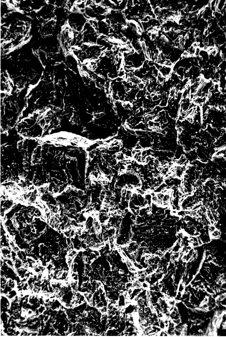
Figure 11. A higher magnification of a non-gassy area from the sample shown in Fig. 10. There is a complete lack of a shear (cup and cone) type of failure. 500X.
