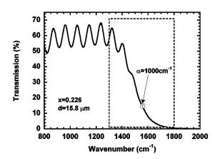
FIG. 1. Room temperature IR transmission spectrum from an arbitrary location on the HgCdTe/CdZnTe epilayer under study. The dotted line indicates the turn-on region of interest for this study, and the  $\alpha = 1000 \text{ cm}^{-1}$ point on the curve is indicated by an arrow.
