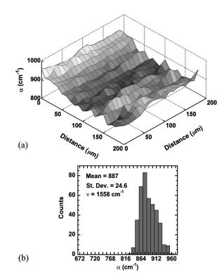
FIG. 3. Plot of (a) absorption coefficient extracted from transmission spectra at a fixed wavenumber of  $\nu = 1558 \text{ cm}^{-1}$  for a 200  $\mu \text{m} \times 200 \ \mu \text{m}$  area and (b) corresponding histogram.
