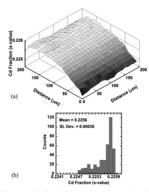
FIG. 4. Plot of (a) HgCdTe composition extracted from the  $\alpha$  = 1000 cm<sup>-1</sup> location on fitted transmission spectra for a 200  $\mu$ m × 200  $\mu$ m area and (b) corresponding histogram.
