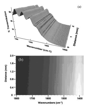
FIG. 2. IR transmission spectra near the turn-on for line scans covering a distance of 2 mm with 10  $\mu$ m spacing. Plots are shown in (a) three dimensions and (b) as a contour plot.
