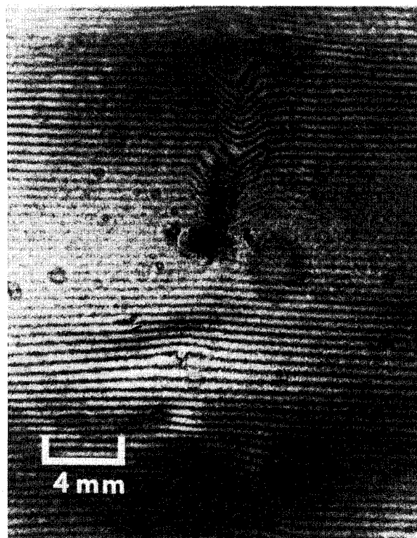
FIG. 6. Interferogram of exploding lithium wire plasma at t_0 + 2.1 \mu\text{s} .
