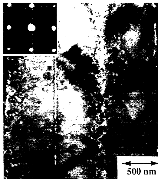
FIG. 7. Cross section TEM micrograph and TED pattern near the top of a 2 \mu\text{m} Mo film deposited at 34 nm/min. The TEM micrograph shows the columnar microstructure of the film. The TED pattern corresponds to a \langle 200 \rangle zone axis pattern for a bcc material, and was obtained by placing an aperture about \approx 8 of the columns.
