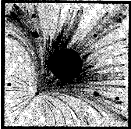
FIG. 29. Same as in Fig. 28, but flow space doubled. Lessened refraction shows that the larger the flow spacing, the less the effect of spacing inequalities.
