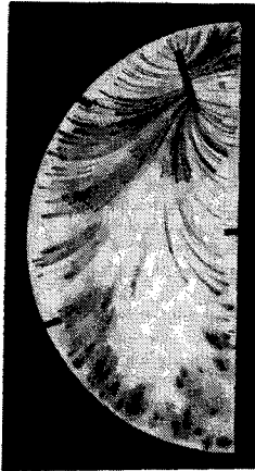
FIG. 34. Open-edge slab, small narrow sectorial sandbed used as sink. Solving for Foucault (damping) currents in a round disk, rotating through a flux piercing the disk.
