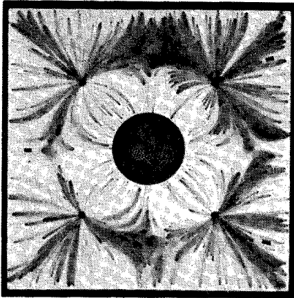
FIG. 11. Square slab, open edge. Four small equal sinks, large round central source.
