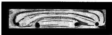
FIG. 19. As in Fig. 18, but sources and sinks displaced downward. The particles are MnO_2 precipitate.
