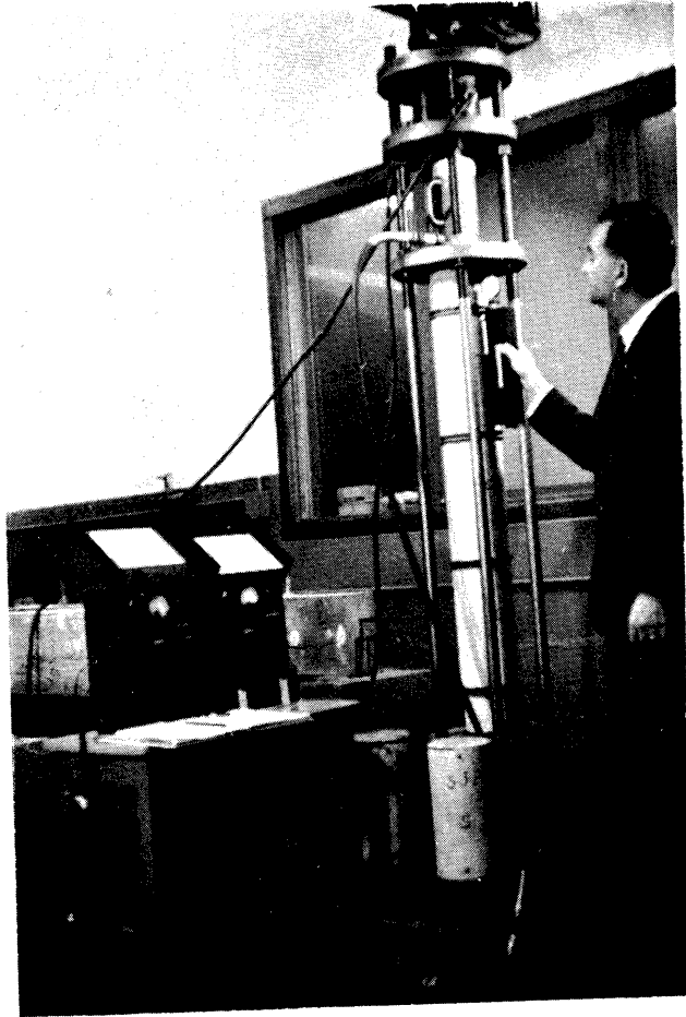
Figure 4.8. Test Rig for Determining Creep of Concrete Under Load.
